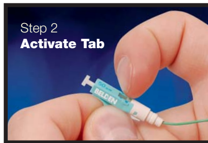
2. Using your index finger, slide the connector's switch-like activator tab toward the fiber to be terminated to bring about the splice/crimp
